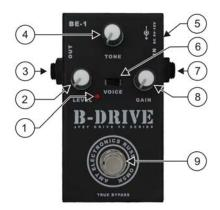
Drive Series Effects are easy to handle and require minimum adjustments.
